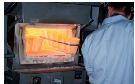
Figure 2, unloading the Fire Assay furnace
